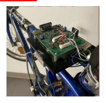
So far, our team has been able to develop an autonomous bicycle that is capable of navigating and balancing itself. While others have developed autonomous bicycles using gyroscopes or reaction wheels, our mission is to reduce weight and manufacturing costs by balancing our bike only through the steering control of the front wheel.
